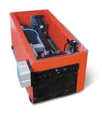
The P30/50 pneumatic cable stripping machine is designed for removing the outer insulation of cables up to 30mm in diameter.
